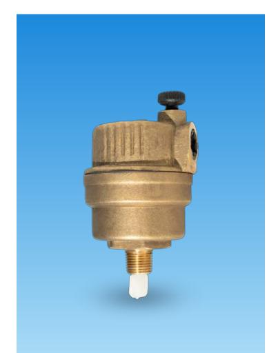
The FLO FAB Automatic Air Vent series AA is designed for continuous air venting in hot and chilled water systems. When used to protect coils, it is best located on the supply side of the coil to prevent air from entering the coil and requiring a service call to vent the air. The unit is best located where pipe velocities are reduced. An ideal location is directly in the body ot a «Y» Strainer. The strainer screen breaks and collects bubbles which are vented by
